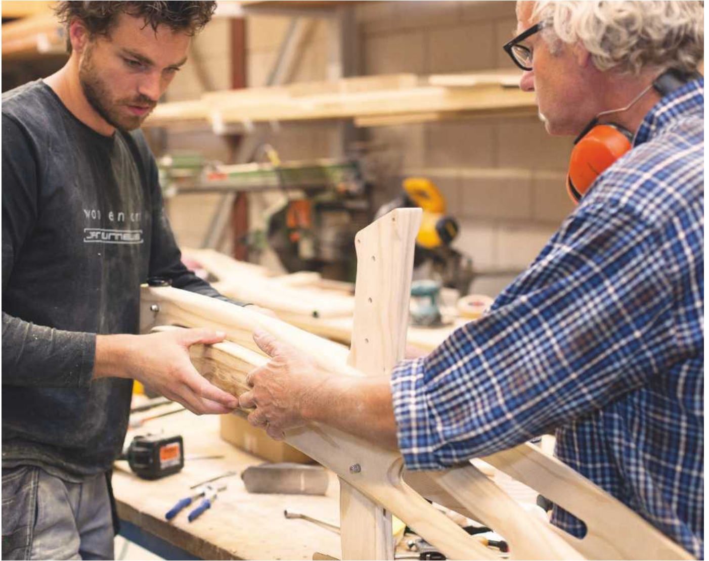
The Bough Bike frame under construction is made from French oak
